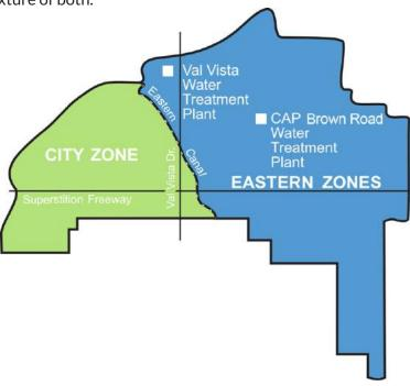
**City Zone** - Salt and Verde River water from the Salt River Project (SRP) supplies water delivered in the City Zone. This water is treated at the Val Vista Water Treatment Plant by using conventional filtration, fluoridation, and disinfection using chlorine dioxide and chlorine before entering into Mesa's water distribution system. Approximately 26% of all the water served to Mesa's customers in 2017 came from this source.
