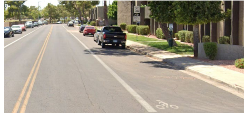
Shared bike and parking lane no longer meets the latest MUTCD Guidance
